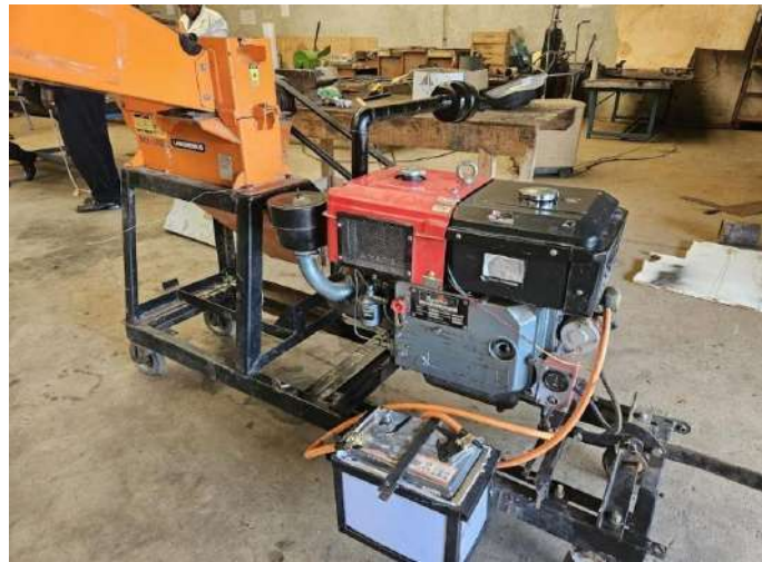
Figure 2: MCTn® machine (Laboremus, Campina Grande, Brazil) used for crushing cactus.
