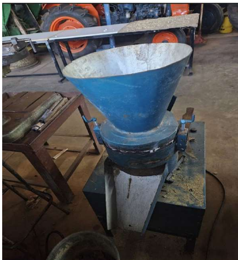
Figure 5: Pelleting machine used for pelleting the mixture into cactus-based pellets.
