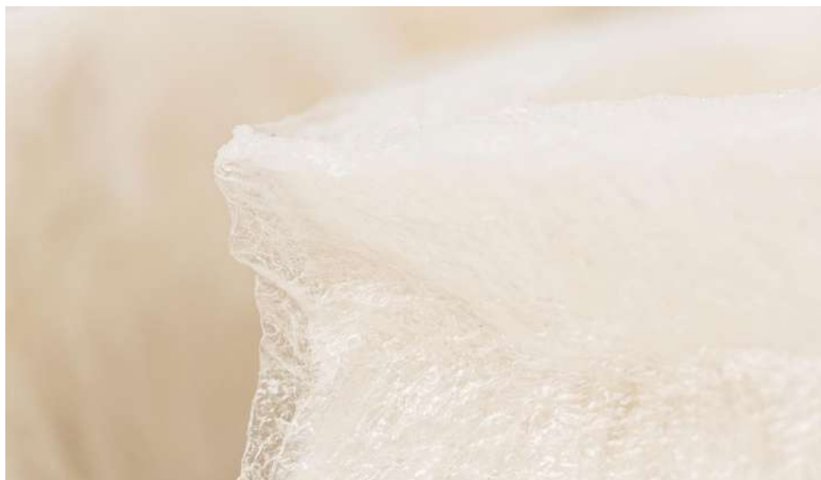
Figure 3: Surface microtexture: Fibrous, lightweight cell structure from air-drying gives a natural tactility.
