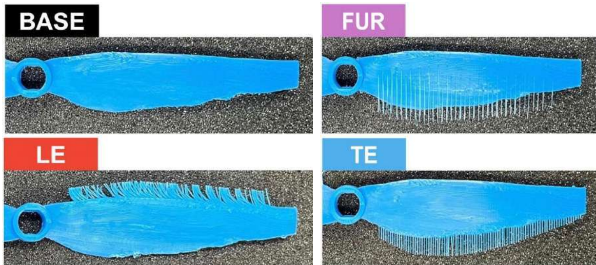
Figure 2: Photos of printed AeroFeather propeller blades compared to a clean BASE blade without any modifications.
