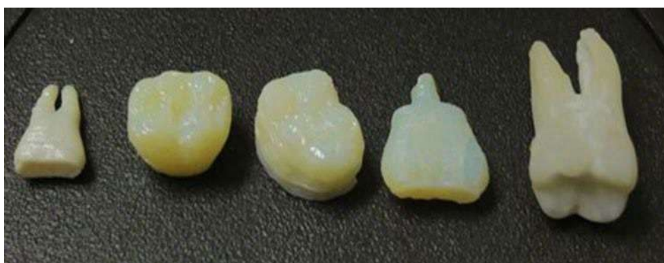
Figure 2: DIW 3D printed nanostructured YSZ dental components.
