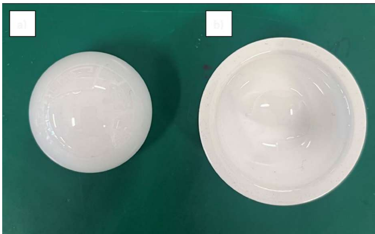
Figure 4: DLP 3D printed ceramic hip implants: a) Femoral Head and b) Acetabular Cup.
