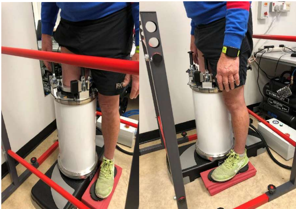
Figure 6: PCAD transtibial residual limb shape capture clinical investigation.
