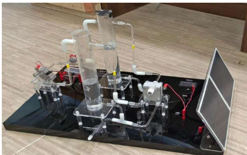
Figure 4: Closed-loop schematic of compact solar-driven hydrogen fuel cell system.
