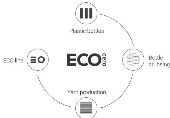
Figure 1: Fabrication process of ECOcero sound-absorbing PET panels (Source: ECOcero https://ecocero.com/en/ ).
