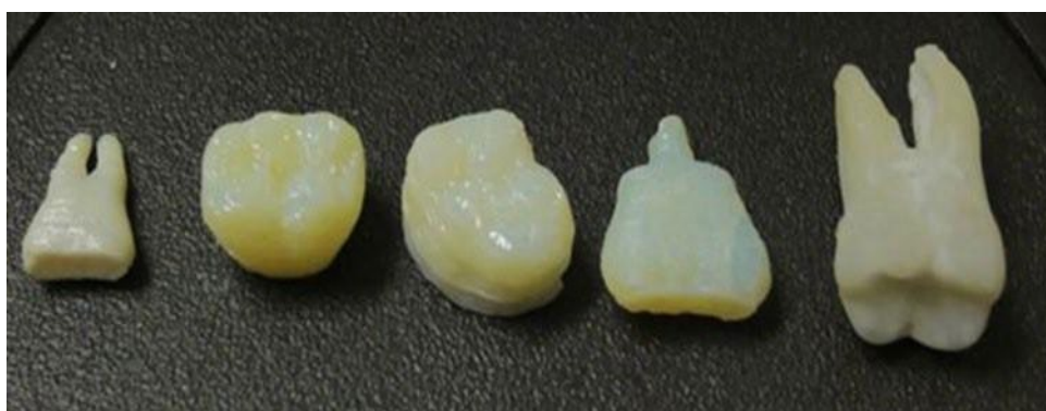
Figure 2: DIW 3D printed nanostructured YSZ dental components.
