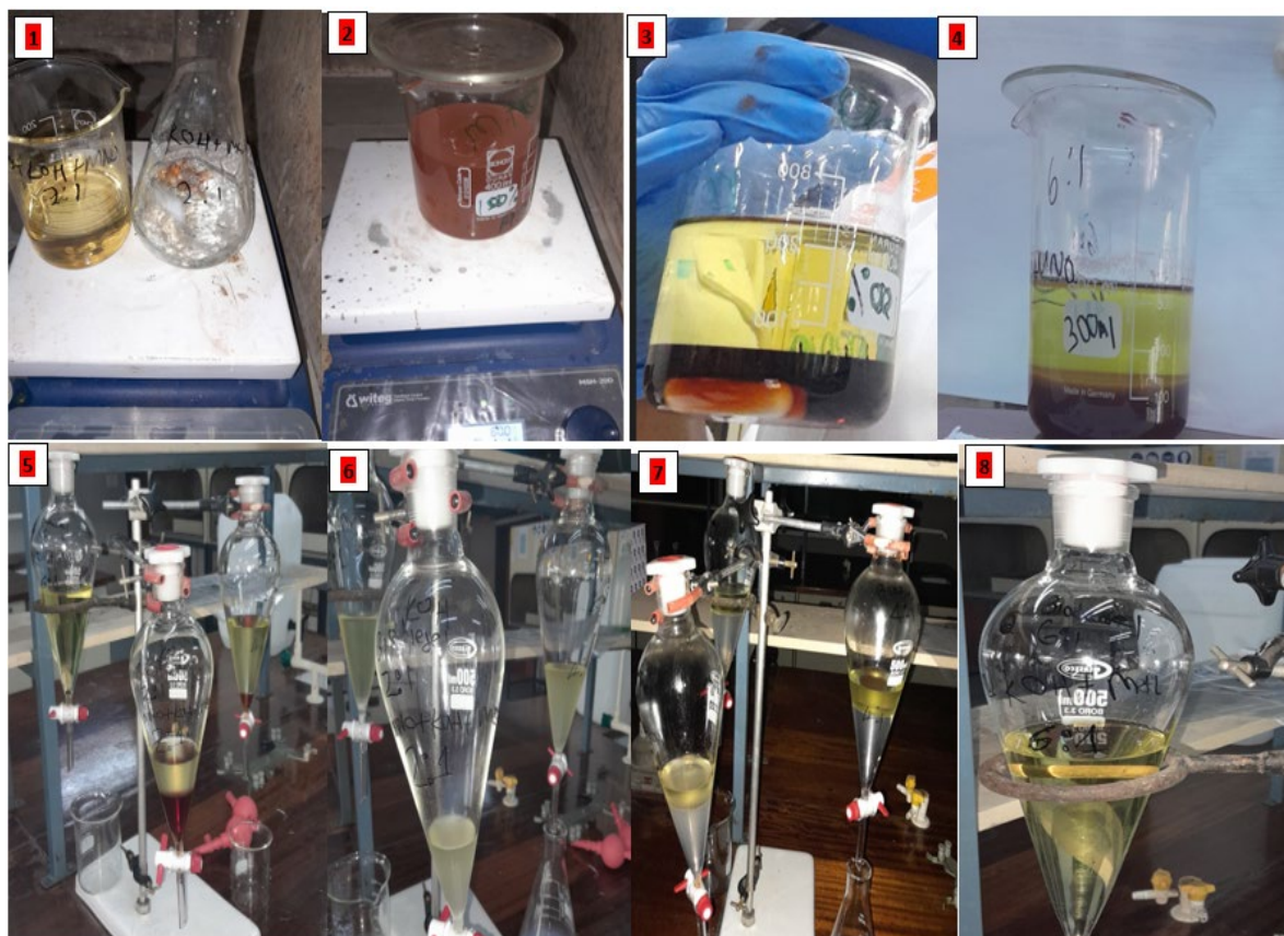
Figure 1: Synthesis and phase separation of macadamia nut biodiesel with reagent preparation and mixing (1–4), followed by phase separation of the reaction mixture (5–8).
