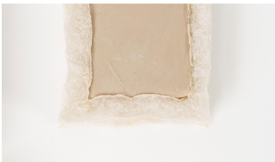
Figure 2: Cast rectangular pad: Air-dried pad for lining/spacing; dimensions are set by the mould family.
