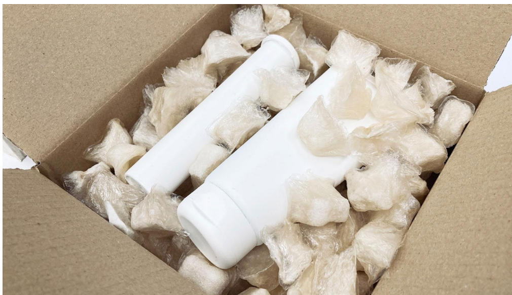
Figure 4: Loose-fill “packing peanuts” in use. Seaweed foam surrounds products and fills voids in a standard e-commerce box.
