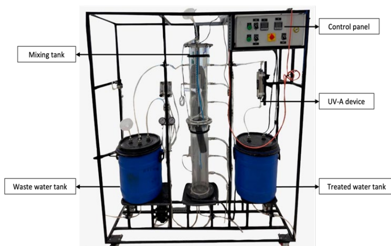
Figure 1: Experimental setup prototype showing the circulation system, mixing tank, and UV/solar integration.
