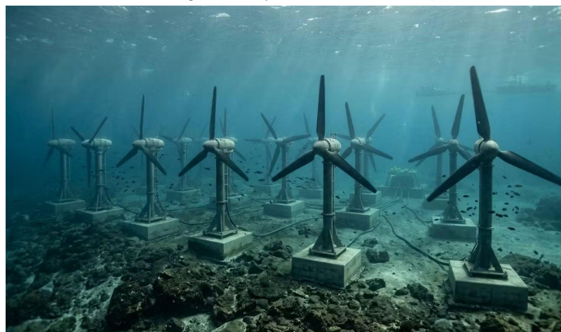
Figure 2: An image of a traditional hydrokinetic CEC array. Notice the short turbine blades relative to a traditional terrestrial wind turbine.
