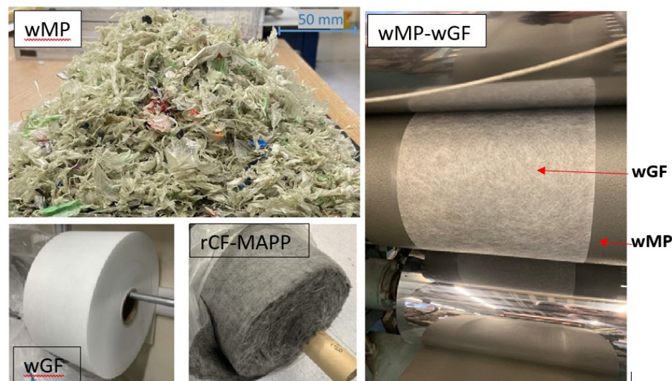
Figure 1: Waste mixed plastics (wMP), waste glass nonwoven mat (wGF), and wMP-coated wGF mats.
